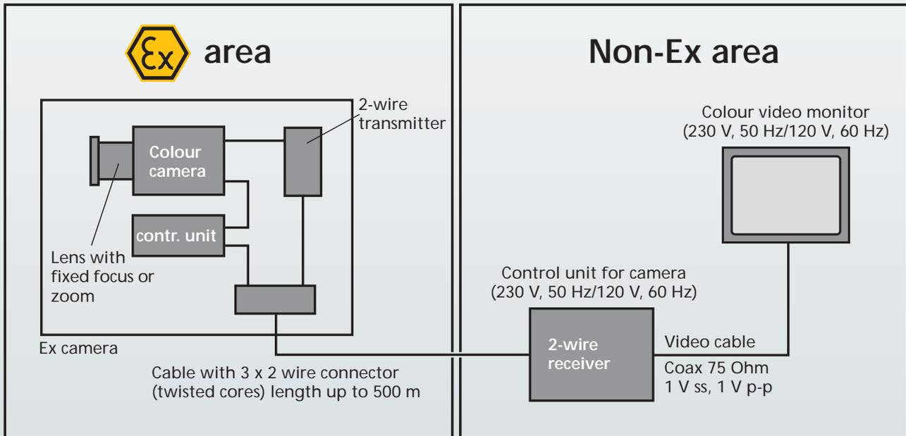
Connecting the Ex camera to a Monitor and/or PC
